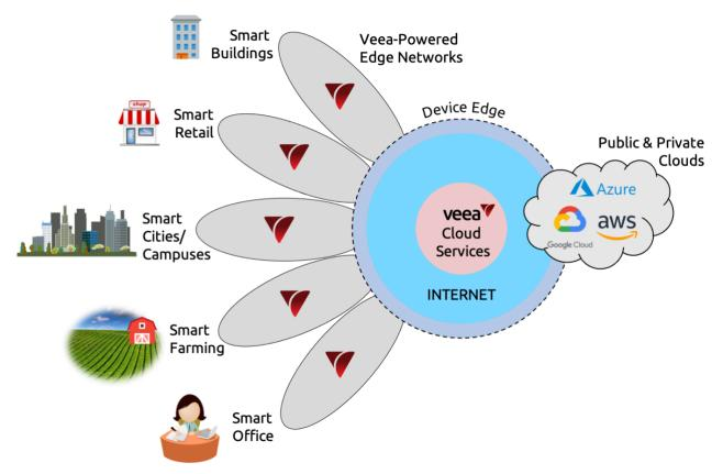
Veea's proprietary vMesh technology is used to create the self-organizing, resilient, route-optimized hybrid wired/wireless network over which data is communicated between individual VeeaHubs (the nodes of the network). Veea's vBus technology is the abstraction layer that allows applications running anywhere on the mesh to work with IoT devices and storage anywhere on the mesh.
